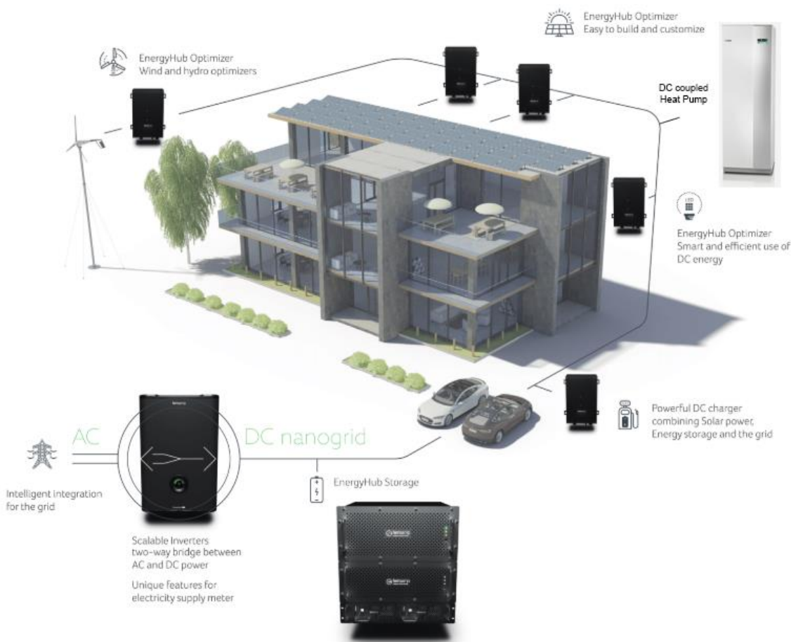
Figure 4. Illustration of how the DC coupled heat pump can be integrated with the Ferroamp DC nanogrid
