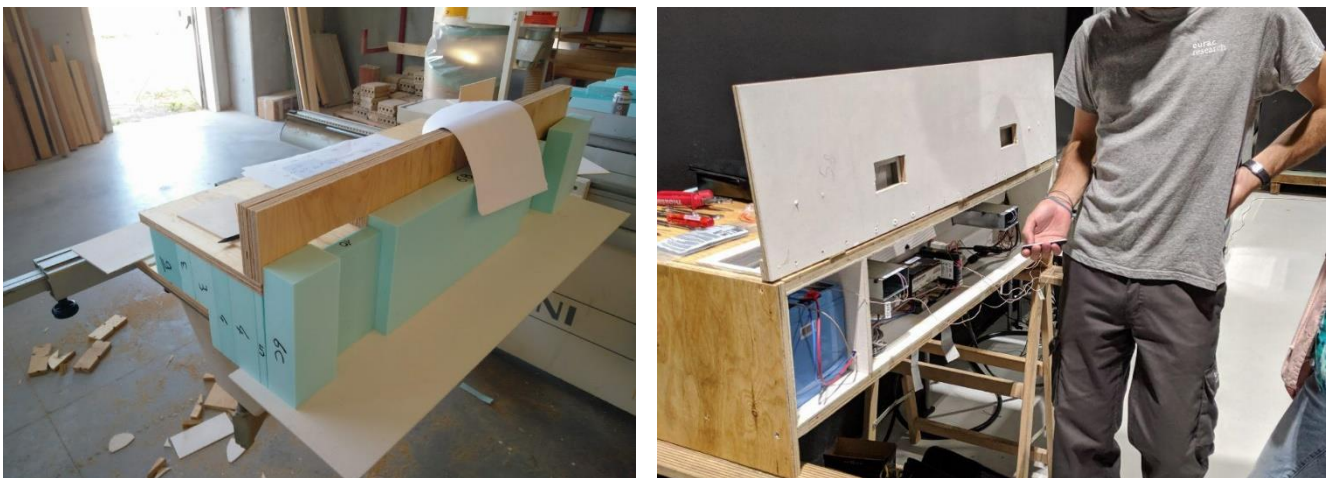
Figure 13. Mock-up for electrical components overheating tests (Source: Eurofinestra)
