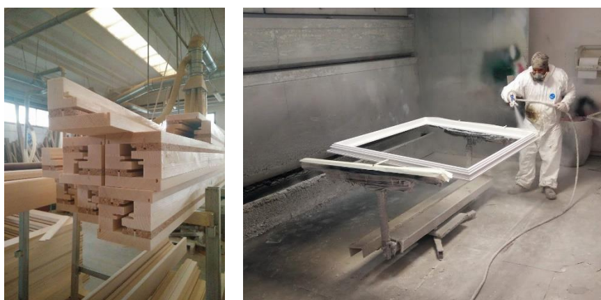
Figure 7. Window frame manufacturing (Source: Eurofinestra)
