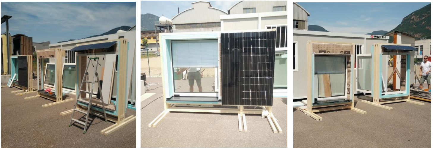
Figure 12. Mock-ups installation in outdoor laboratory (Source: Eurofinestra)
